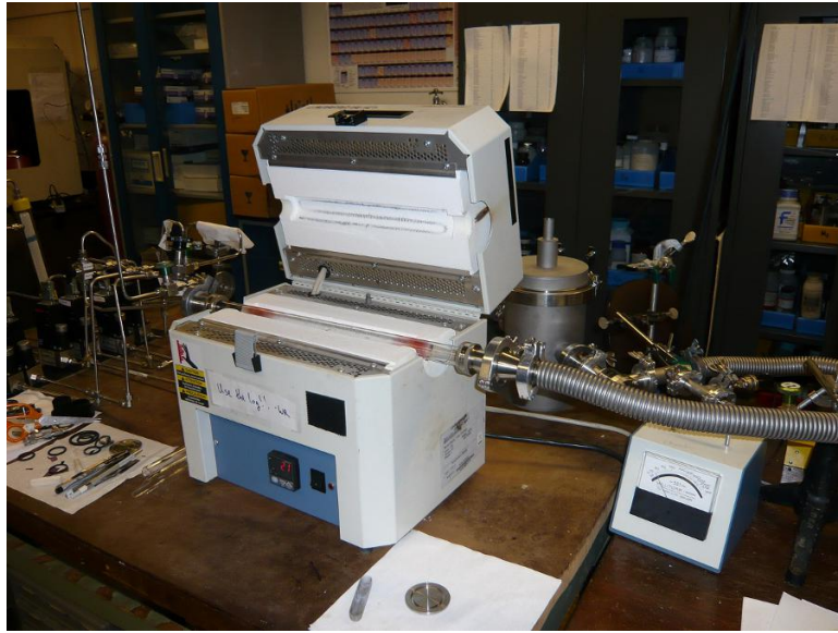
Figure 3.3: A picture of the carbon CVD system used for graphene and carbon nanotube synthesis. A quartz tube sitting in a furnace holds the growth substrate; gases enter the tube through the steel lines on the left and exhaust to a vacuum (or bubbler, for atmospheric pressure recipes) on the right.
