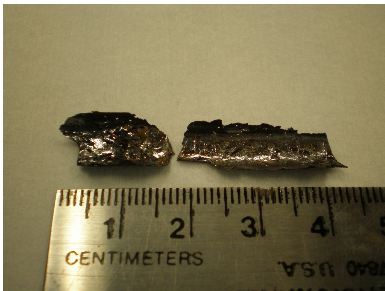
Figure 5.16: Boule of tin sulfide grown with the Bridgman technique. Most of the material appears amorphous, but large flakey brown crystals are also present.
